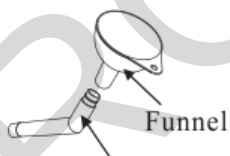
Funnel Lubricating oil pipe
