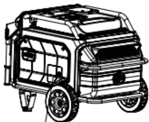
Oil service door
